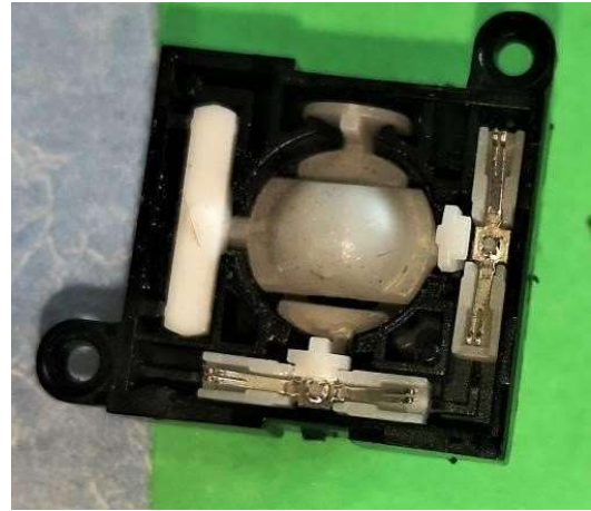
Photo 16 Dust in the internal structure
